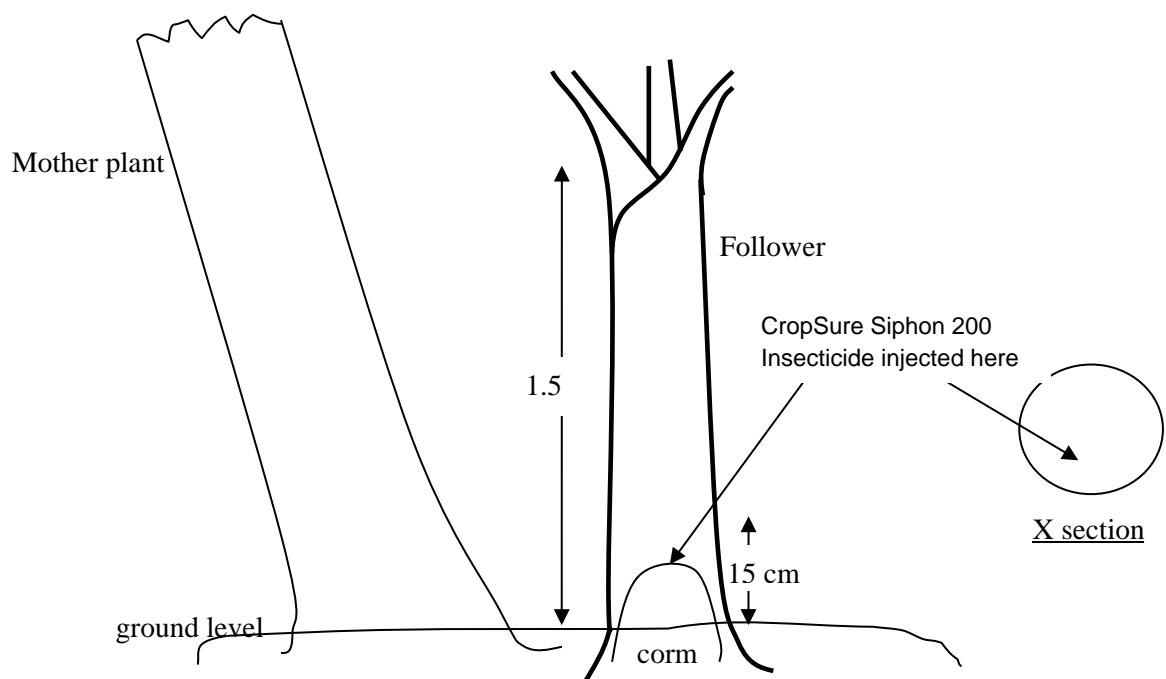
**Stem Spray:** The trunk spray should be applied with a full cone nozzle directed at the base of the stem and up to a height of 300 mm, so that it covers around 40% of that area of the stem. The spray should be calibrated so it delivers 10 mL of mixture per stem.
